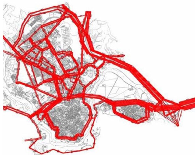
Daily Average Intensity Map in the Road System only elaborated for motor traffic. Source: Plan de Movilidad Urbana Sostenible de Toledo, 2007.
